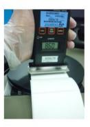
Measured the static charge build-up with the label attached to the reel -measurement reading was 98V –which is good (Criteria is <100 V)
